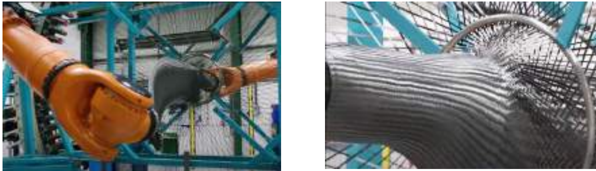
Figure 28.19 Radial braiding technique
